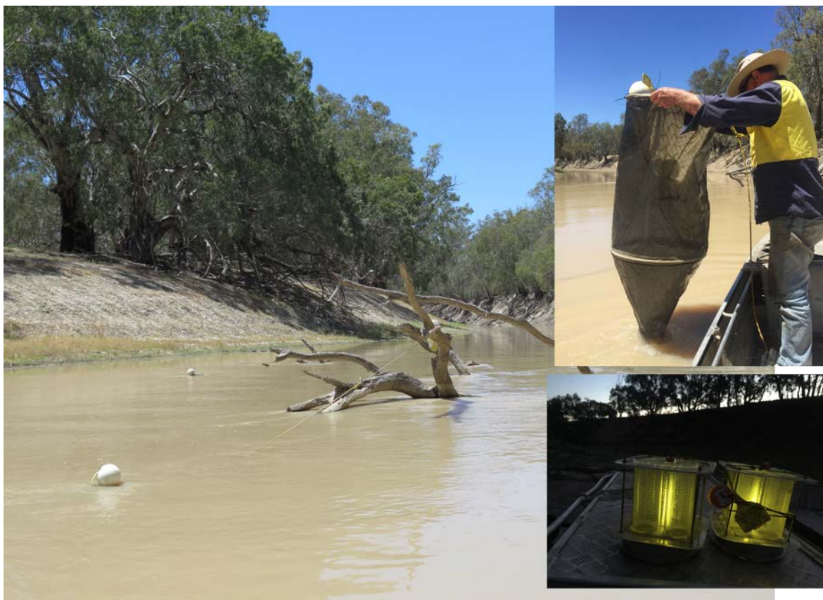
Figure 4. Examples of the larval nets and traps used in Yanco-Colombo Creeks in 2017. A drift net suspended from a snag (in the Darling River, main image). The contents are sieved and collected as a sample, preserved and identified in the laboratory (top right). Light traps prior to deployment showing the light emitted from glow sticks that attract fish larvae (bottom right). Three of each of these nets and traps were deployed overnight on each sampling occasion at nine sites in Yanco-Colombo Creek and two sites in the Murrumbidgee River from 20 September to 9 December 2017. Images: C. Sharpe
